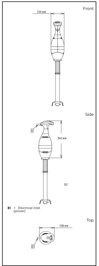
Electric Supply voltage: 220-240 V/1 ph/50/60 Hz Electrical power, max: 0.65 kW 0.65 kW **Total Watts:** Key Information: External dimensions, Width: 138 mm External dimensions, 120 mm Depth: External dimensions, 340 mm Height: **Shipping weight:** 3.7 kg
